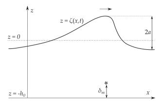
**Fig. 1.** Sketch of the Cartesian coordinate system: *x* is the horizontal axis along which waves propagate and *z* points vertically upwards, with z = 0 being the mean water level and  $z = -h_0$  the distance to the bottom. The wave amplitude is noted *a* and  $\delta_m$  represents the distance to the bottom at which the pressure is measured.
