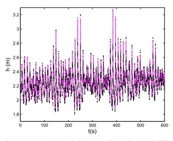
**Fig. 6.** Reconstruction of water depth time series of waves observed in the field. Cut-off frequency  $f_c = 1$  Hz,  $\bar{h} = 2.25 m$ ,  $\delta_m = 0.69 m$ . dot: direct acoustic measurement of h; magenta line:  $h_{\text{SNL}} = \bar{h} + \zeta_{\text{SNL}}$ , Eq. (13).
