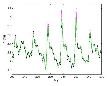
**Fig. 7.** Reconstruction of water depth time series of a group of waves observed in the field. Cut-off frequency  $f_c = 1$  Hz,  $\bar{h} = 2.25 m$ ,  $\delta_m = 0.69 m$ . dot: direct acoustic measurement of *h*; green line:  $h_{\rm SL} = \bar{h} + \zeta_{\rm SL}$ , Eq. (12); magenta line:  $h_{\rm SNL} = \bar{h} + \zeta_{\rm SNL}$ , Eq. (13). (For interpretation of the references to colour in this figure legend, the reader is referred to the Web version of this article.)
