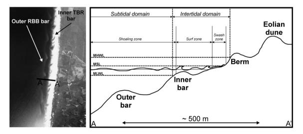
Fig. 2. Aerial photograph (IGN) of a section of the Aquitanian Coast displaying a double bar system, with typical Aquitanian Coast beach profile.
