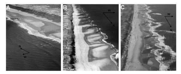
Fig. 4. Aerial photographs of different intertidal bar morphology during low-tide, Aquitanian Coast. (A): Typical LTT morphology; (B) regular TBR morphology; (C): TBR morphology with rip channels oriented in no preferred direction.
