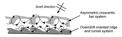
Fig. 9. Asymmetric behaviour of the outer nearshore crescentic bar and inner bar LTT morphology as a function of wave-induced currents, circulation cell patterns and wave angle (Castelle et al., 2005).
