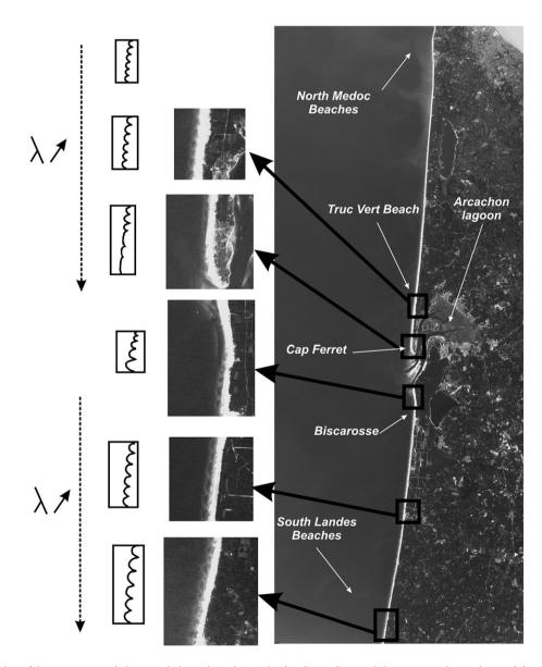
Fig. 12. Variation of the outer crescentic bar morphology along the Aquitanian Coast. Crescentic bars are not observed around the Arcachon lagoon inlet where tidal currents are intense, and the outer bar alongshore averaged wavelength  $\Lambda$  slightly increases to the south, after Castelle (2004).
