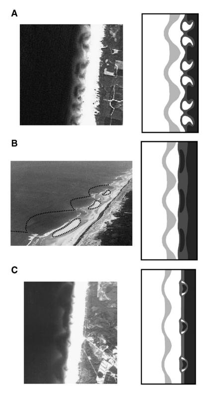
Fig. 10. Evidence of strong morphological coupling between the inner and outer bars (Castelle, 2004). A: Satellite SPOT image (15/10/2001@CNES UMR EPOC 5805); B: Aerial photograph (1999); C: Aerial photograph (IGN, 1978).
